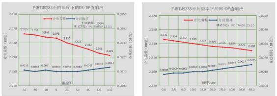
Excellent frequency stability: the material has stable dielectric constant and loss within 0.5~40GHz frequency, maintaining ultra-low loss value to meet the design requirements at different frequencies;
