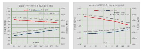
◆ Excellent frequency stability: the material has stable dielectric constant and keeps low loss value in the frequency of 0.5 ~20GHz, which meets the design requirements under different frequencies;
