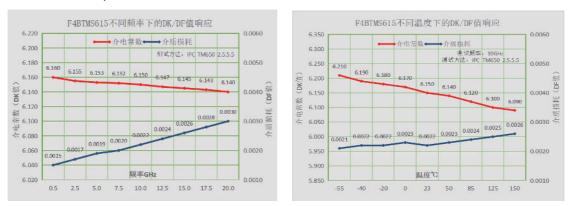
◆ Excellent frequency stability: the material has stable dielectric constant and keeps low loss value in the frequency of 0.5~20GHz, which meets the design requirements under different frequencies;
