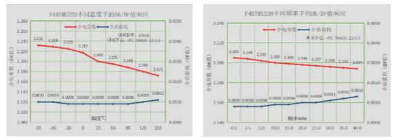
Excellent frequency stability: the material is stable in terms of dielectric constant and loss within 0.5 to 40 GHz frequency, maintaining ultra-low loss values to meet the design requirements at different frequencies;
