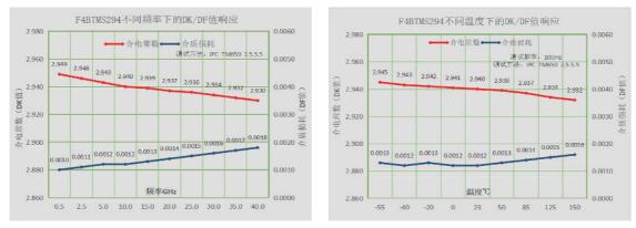
• Excellent frequency stability: the material has stable dielectric constant and loss within 0.5~40GHz frequency, keeping low loss value to meet the design requirements under different frequencies;
