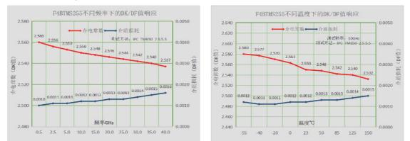
• Excellent frequency stability: the material has stable dielectric constant and loss within 0.5~40GHz frequency, maintaining low loss value to meet the design requirements at different frequencies;
